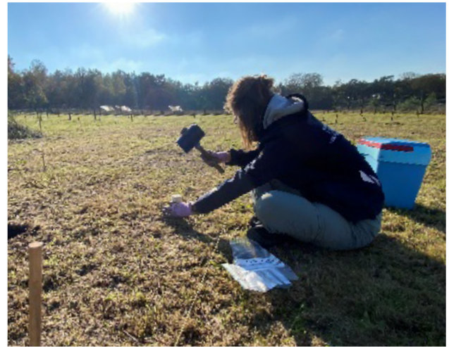
Fig. 18: Sampling with hammer and pre-cut PVC soil core.
