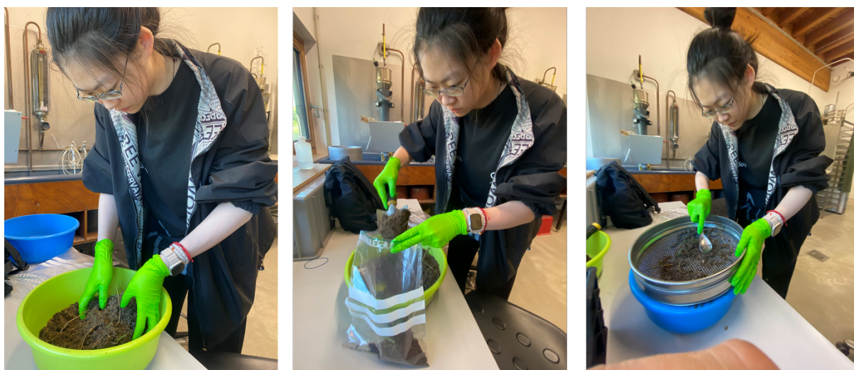
Fig. 37: Mixing and sub-sampling nematodes. Sieve remaining sample through 2 mm mesh and sub-sample for physico-chemical and eDNA samples.
